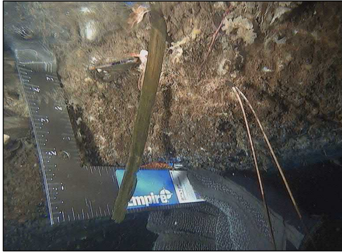
Figure 59 - Relative Measurement of Loss of Cross-Sectional Area on Polystyrene Billet
