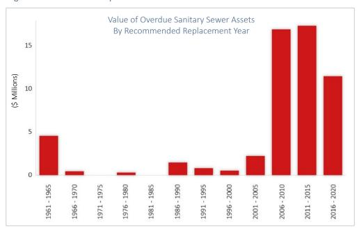
Figure 26: Past Due Sanitary Sewer Assets
