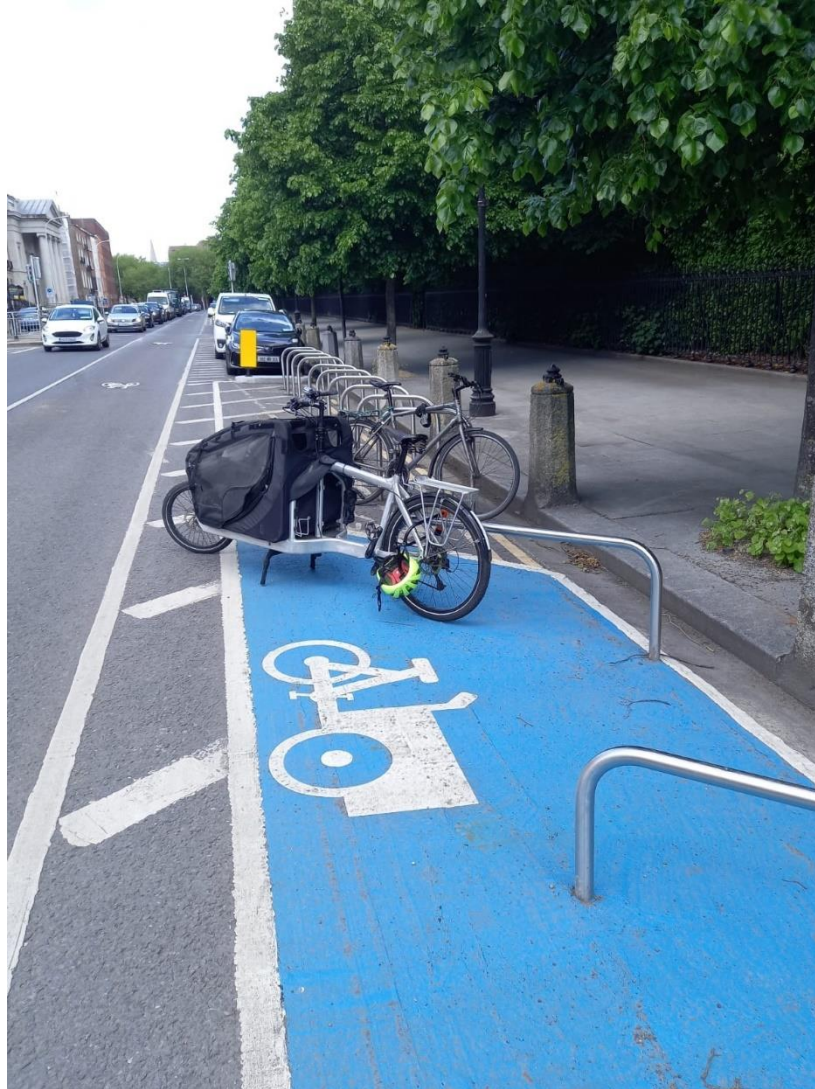
Example of short-term (non-standard) oversized bicycle parking in Dublin, which provides extra space for larger bikes and are delineated with paint to make it easier for users to find. Image credit: Dublin City Council
